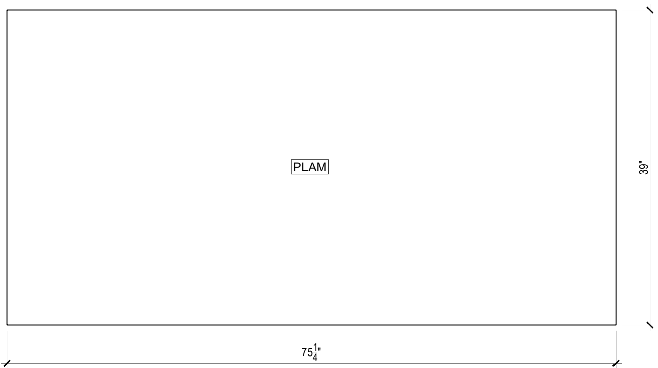
9 STORAGE BENCH -TOP VIEW Scale: 1"=1'-0"
